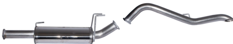
76MM SS TAIL PIPE PERF SS IS1250
